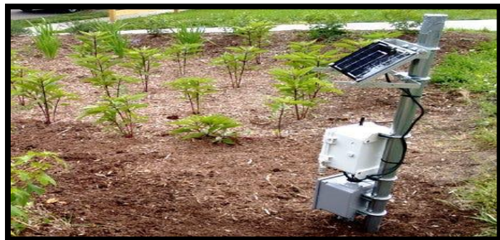
Figure 5-19 Soil Moisture monitoring system
